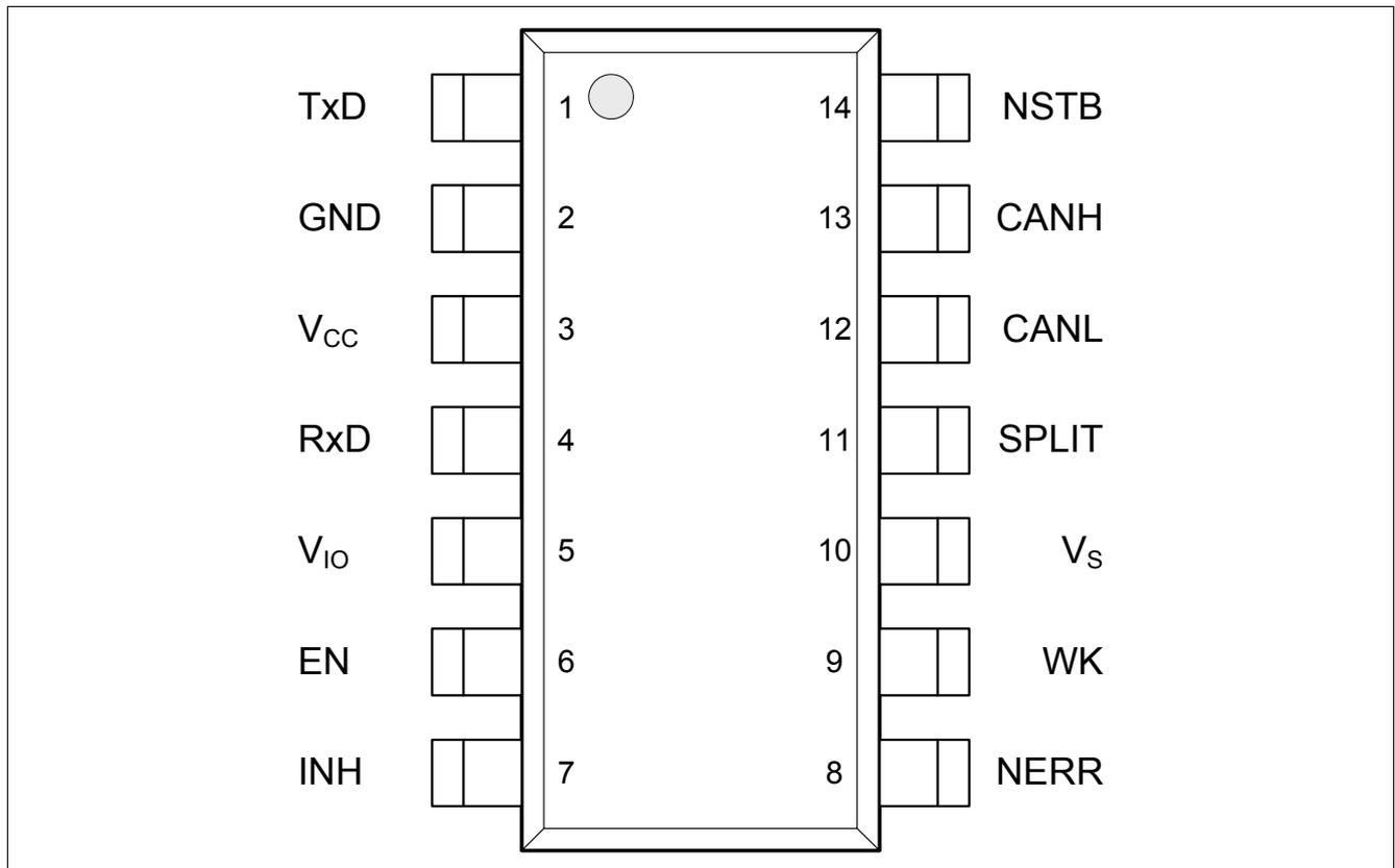
Figure 2 Pin Configuration
