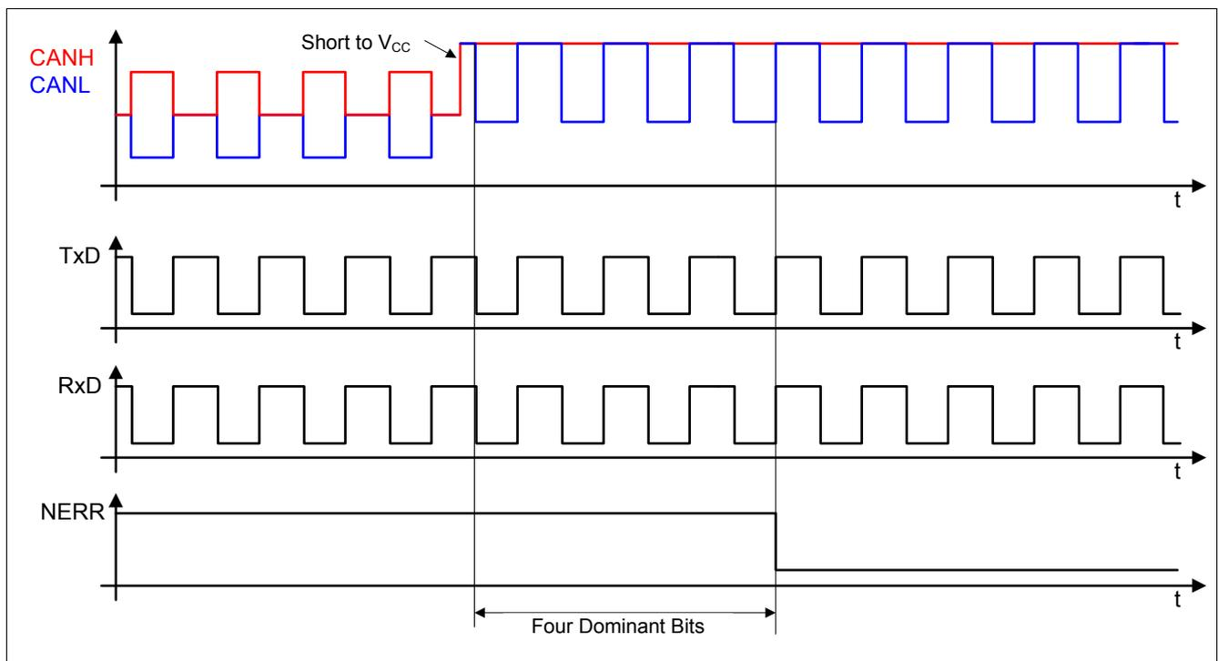
Figure 9 CAN Bus Failure CANH short to  $V_{CC}$ <sup>1)</sup>
